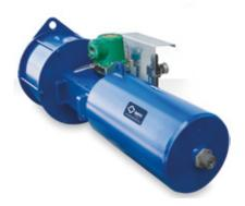
ALGA-ALGAS pneumatic scotch yoke actuators are suitable for quarter-turn valves up to the largest sizes, thanks to an efficient design and to high break-out torque. The QA version with damper performs fail stroking in less than 1 second.
